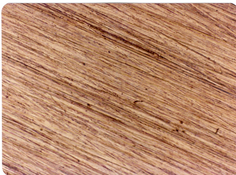
Figure 6. Carbon steel (AISI 1020) polished with 600 SiC paper Mag. x 80.
