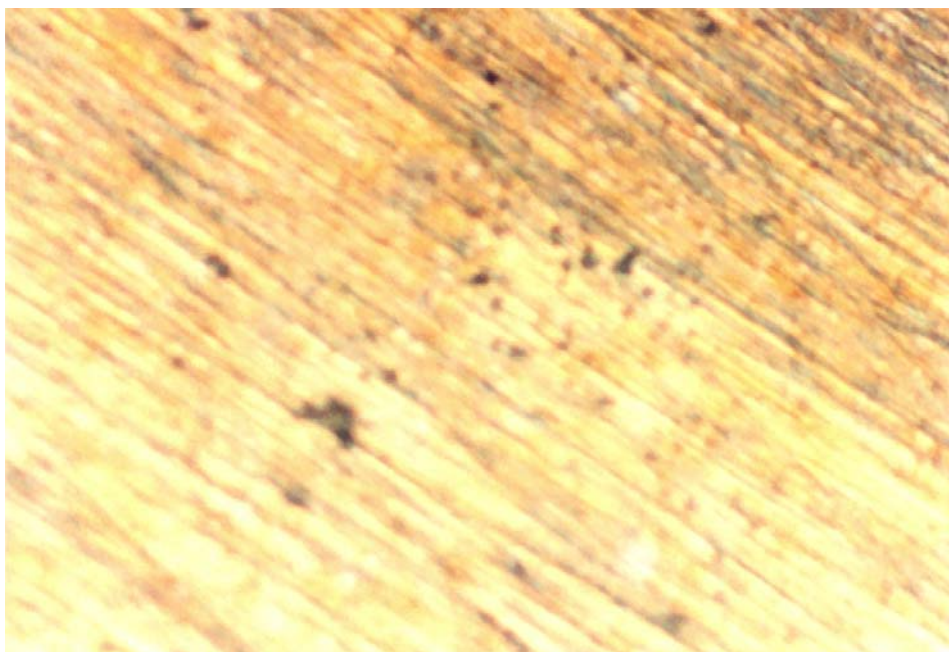
Figure 9. Al-Bronze (C60800) after 60 min exposure is little damaged Mag x 200
