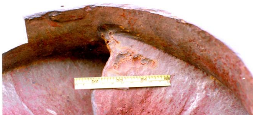
Figure 16. Cavitation erosion-corrosion of a centrifugal pump's impeller
