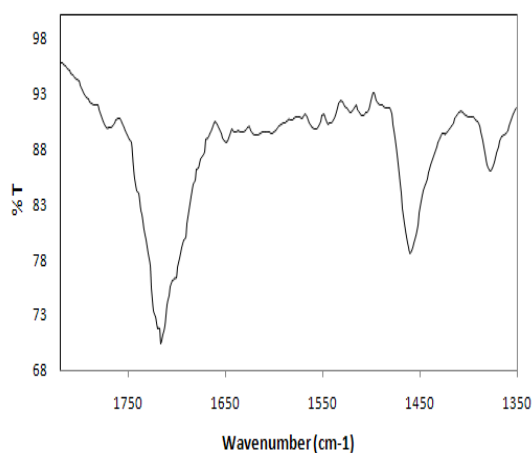
Figure 4. The FTIR result of dried sludge.
