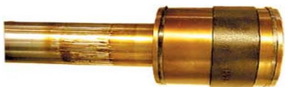
Figure 2. Varnish formation on Inlet Guide Vane (IGV) valve from a gas turbine (Courtesy of Clarus Technologies).
