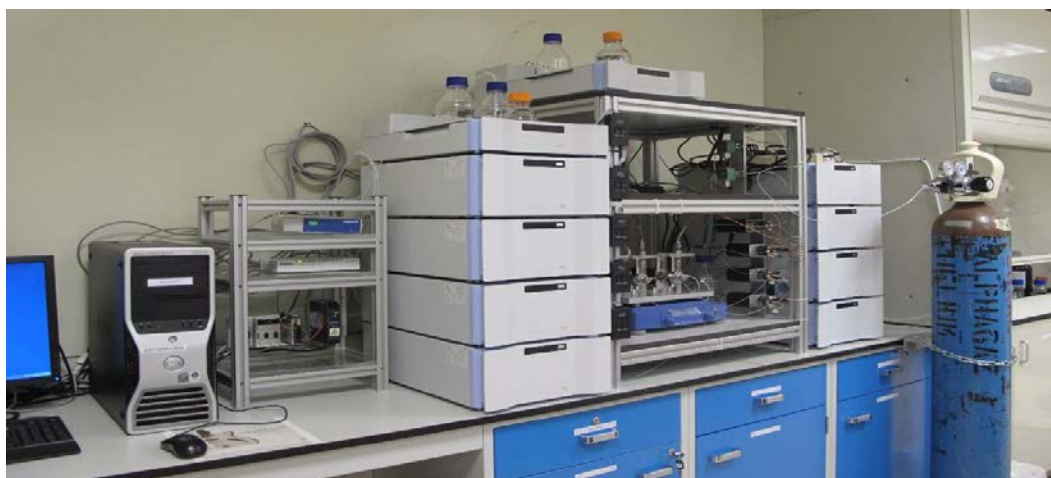
Figure 5. Laboratory process setup displaying HPLC modules, fraction collection, online monitoring, and the HMI system.
