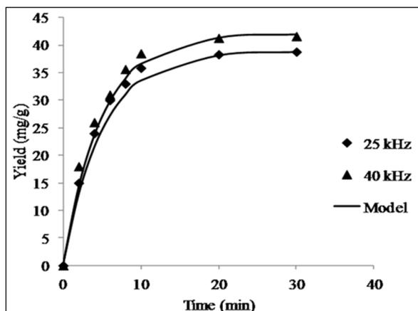
**Figure 4.** Effect of Frequency on extraction yield of GA (Power: 200 W, solvent to solute ratio: 1:30, temperature: 30°C).
