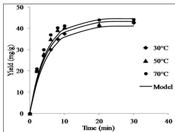
**Figure 5.** Effect of temperature on extraction yield of GA (Power: 200 W, Frequency: 40 kHz, solvent to solute ratio: 1:30).
