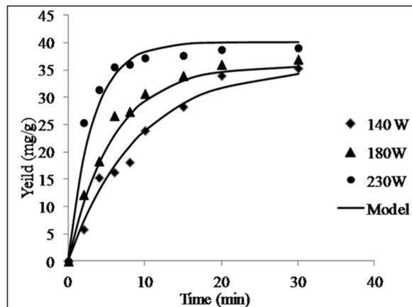
**Figure 3.** Effect of Power on extraction yield of GA (Frequency: 25 kHz, solvent to solute ratio: 1:30, temperature: 30°C).
