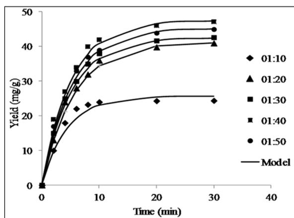
**Figure 6.** Effect of solvent to solute ratio on extraction yield of GA (Power: 200 W, Frequency: 40 kHz, temperature: 30°C).
