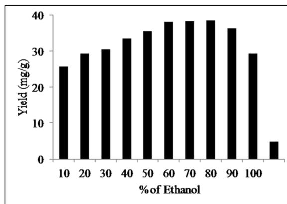
**Figure 1.** Effect of concentration of ethanol on extraction yield of GA (Power: 200 W, Frequency: 25 kHz, solvent to solute ratio: 1:30, temperature: 30°C).
