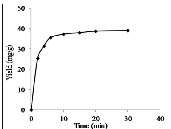
**Figure 2.** Effect of time on extraction yield of GA (Power: 200 W, Frequency: 25 kHz, solvent to solute ratio: 1:30, temperature: 30°C).
