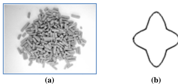
Figure 1. Geometry of quadralobe (a) industrial case, (b) simulation geometry.
