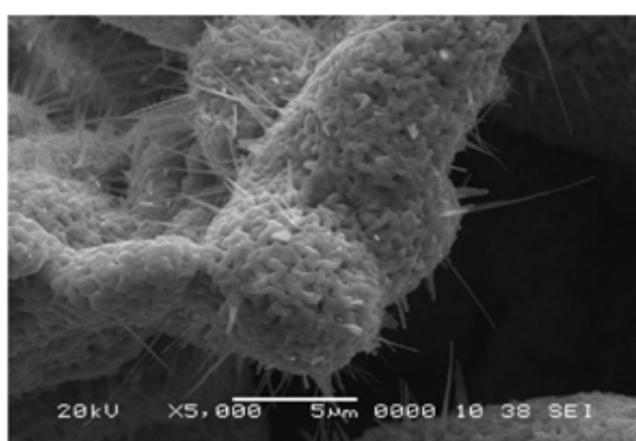
Figure 1. SEM image of direct loaded film at 700 at X5.
