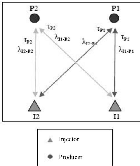
**Figure 2.** A schematic view of a reservoir with 2 injectors and 2 producers which describe the parameters of CRM in this modified approach.
