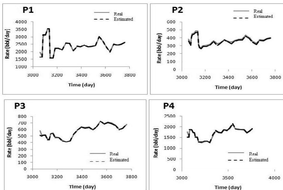
**Figure 8.** Comparison between estimated values of CRM and the calculated values by Eclipse for each producer
