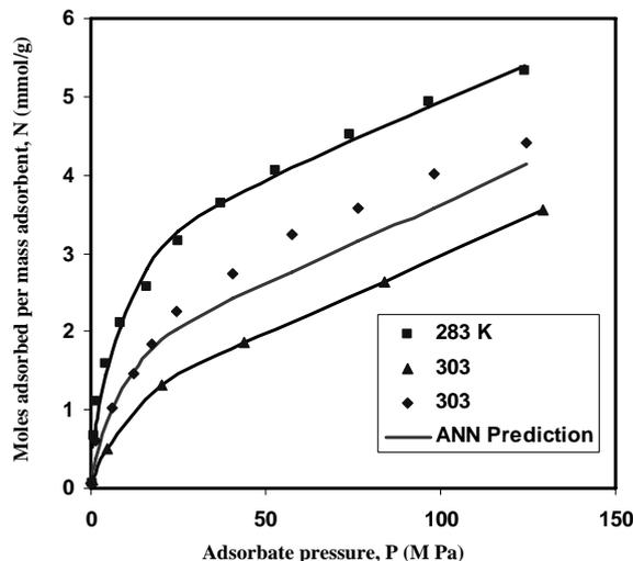
**Figure 6.** Comparison of the experimental adsorption data for  $C_2H_6$ /Ajax Activated Carbon measured by Qiao an Hu[12] with ANN(solid line)
