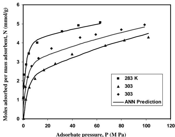
**Figure 5.** Comparison of the experimental adsorption data for  $C_3H_8$ /Ajax Activated Carbon measured by Qiao an Hu[12] with ANN(solid line)
