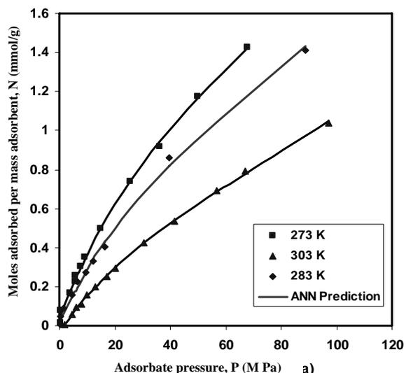
**Figure 4.** Comparison of the experimental adsorption data for  $CH_4$ /Ajax Activated Carbon measured by Qiao an Hu[12] with ANN(solid line)
