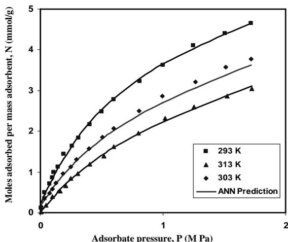
**Figure 3.** Comparison of the experimental adsorption data for  $CH_4$ /activated Carbon measured by Buss[13] with ANN(solid line)
