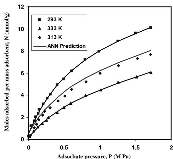
**Figure 2.** Comparison of the experimental adsorption data for  $CO_2$ /activated Carbon measured by Buss[13] with ANN(solid line)
