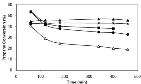
**Figure 2.** Comparison of propane conversion for (●) Pt/Sn/K/La, (■) Pt/Sn/K/Ir, (▲) Pt/Sn/K/Cs, (Δ) Pt/Sn/K/Re and (☆) Pt/Sn/K on  $\gamma$ - alumina supports (WHSV=1.7 h<sup>-1</sup>; T=615°C; H<sub>2</sub>/CH: 0.87).
