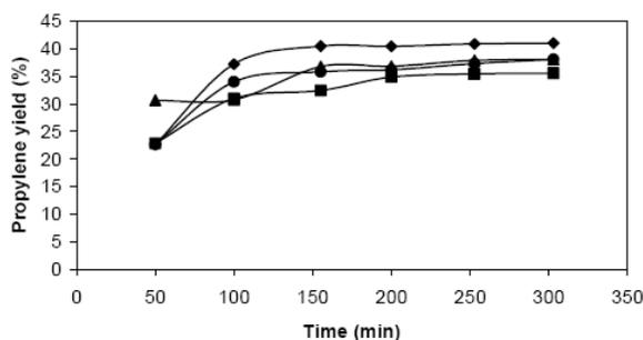
**Figure 7.** Comparison of propylene yield between different Cs concentration on (♦) PtSnK<sub>0.32</sub>Cs<sub>0.32</sub>, (■) PtSnK<sub>0.5</sub>Cs<sub>0.14</sub>, (▲) PtSnK<sub>0.6</sub>Cs<sub>0.04</sub>, and (●) PtSnK<sub>0.62</sub>Cs<sub>0.02</sub> (WHSV=1.7 h<sup>-1</sup>; T=615°C; H<sub>2</sub>/CH: 0.87).
