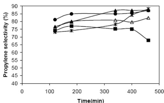
**Figure 3.** Comparison of propylene selectivity for (●) Pt/Sn/K/La, (■) Pt/Sn/K/Ir, (▲) Pt/Sn/K/Cs, (Δ) Pt/Sn/K/Re and (☆) Pt/Sn/K on  $\gamma$ - alumina supports (WHSV=1.7 h<sup>-1</sup>; T=615°C; H<sub>2</sub>/CH: 0.87).
