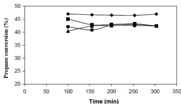
**Figure 5.** Comparison of propane conversion between different Cs concentration on (◆) PtSnK<sub>0.32</sub>Cs<sub>0.32</sub>, (■) PtSnK<sub>0.5</sub>Cs<sub>0.14</sub>, (▲) PtSnK<sub>0.6</sub>Cs<sub>0.04</sub>, and (●) PtSnK<sub>0.62</sub>Cs<sub>0.02</sub> (WHSV=1.7 h<sup>-1</sup>; T=615°C; H<sub>2</sub>/CH: 0.87).
