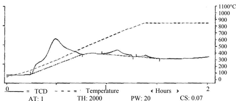
**Figure 1.** TPR spectrum for Pt-Sn-K/Al<sub>2</sub>O<sub>3</sub> catalyst
