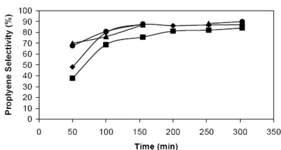
**Figure 6.** Comparison of propylene selectivity between different Cs concentration on (♦) PtSnK<sub>0.32</sub>Cs<sub>0.32</sub>, (■) PtSnK<sub>0.5</sub>Cs<sub>0.14</sub>, (▲) PtSnK<sub>0.6</sub>Cs<sub>0.04</sub>, and (●) PtSnK<sub>0.62</sub>Cs<sub>0.02</sub> (WHSV=1.7 h<sup>-1</sup>; T=615°C; H<sub>2</sub>/CH: 0.87).
