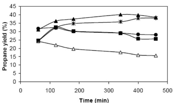
**Figure 4.** Comparison of propylene yield for (●) Pt/Sn/K/La, (■) Pt/Sn/K/Ir, (▲) Pt/Sn/K/Cs, (Δ) Pt/Sn/K/Re and (☆) Pt/Sn/K on  $\gamma$ - alumina supports (WHSV=1.7 h<sup>-1</sup>; T=615°C; H<sub>2</sub>/CH: 0.87).
