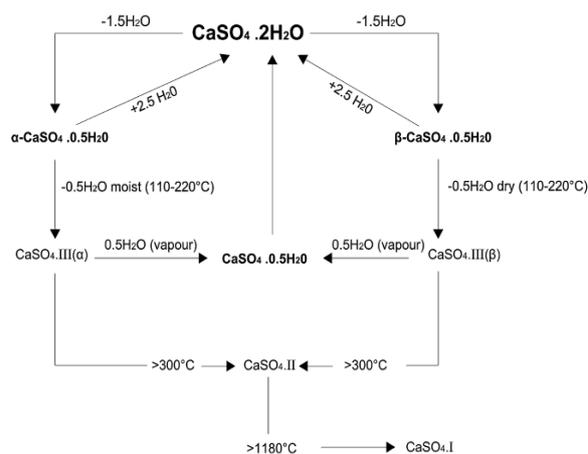
**Figure 1.** Different modifications of  $\text{CaSO}_4 \cdot x\text{H}_2\text{O}$  ( $x = 0.0-2.0$ )
