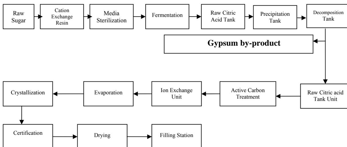
Figure 2. Schematic of the citric acid production process in Kimia Gharb Gostar Industries Company
