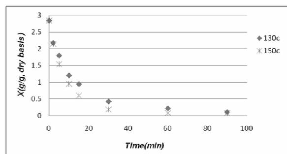
**Figure 3.** Experimental drying curve for sugar beet at 130 and  $150^{\circ}\text{C}$  in a fluidized bed dryer
