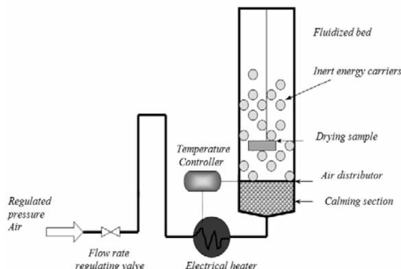
Figure 2. Schematic diagram of the experimental column
