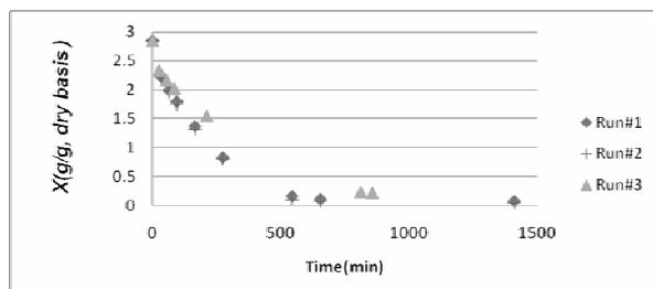
**Figure 4.** Experimental drying curve of sugar beet in the freeze dryer (at -95°C and 10 mtorr)
