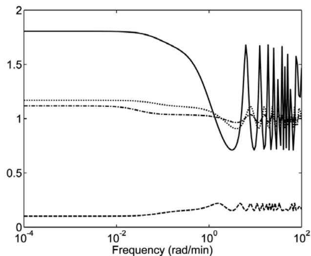
**Figure 2.** Frequency-dependent behavior of 1,1-element of RGA ( $\lambda_{11}$ ) for the selected structures (Waller *et al.*, 1988). — *LV*; --- *DV*; ...  $(D/(L+D))V$ ; -.-  $(D/(L+D))(V/B)$ .
