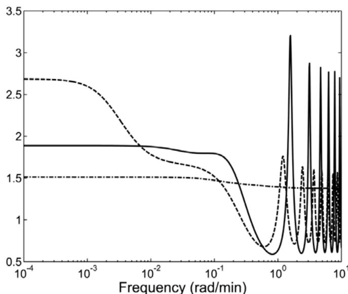
**Figure 4.** Frequency-dependent behavior of 1,1-element of RGA ( $\lambda_{11}$ ) for three different columns using the LV-structure (Georgiou *et al.*, 1988). — Column A ( $L/D = 0.96$ ); --- Column B ( $L/D = 1.19$ ); -·-·- Column C ( $L/D = 0.70$ ).
