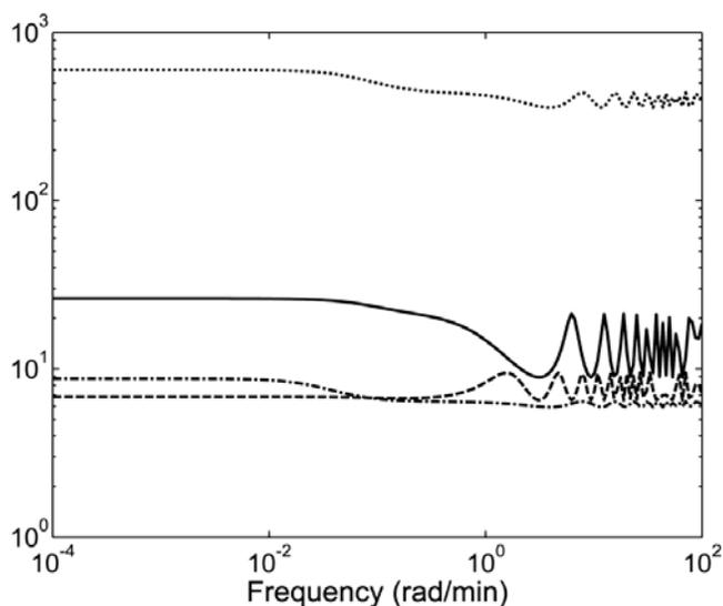
**Figure 1.** Frequency-dependent behavior of condition number ( $\gamma$ ) for the selected structures (Waller *et al.*, 1988). — *LV*; --- *DV*; ...  $(D/(L+D))V$ ; -.-  $(D/(L+D))(V/B)$ .
