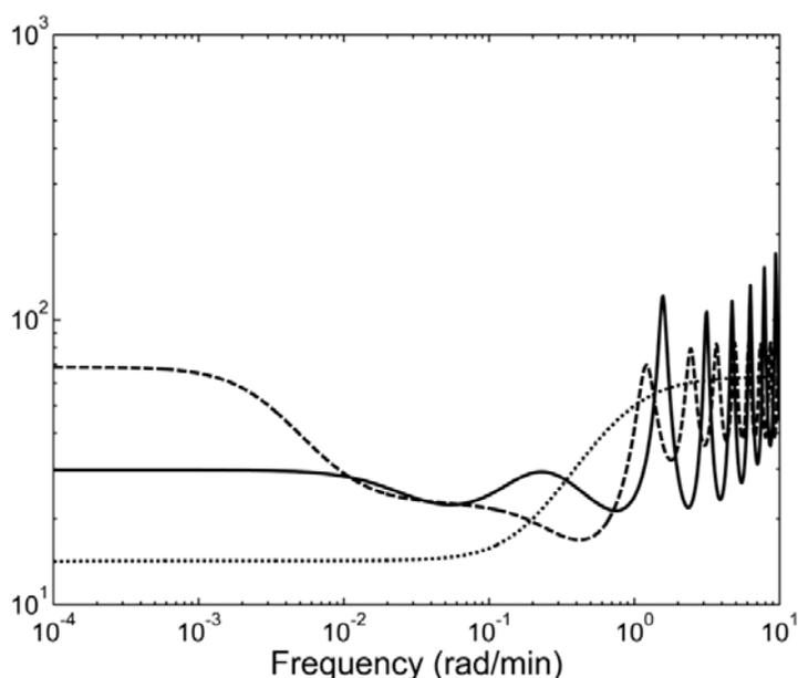
**Figure 3.** Frequency-dependent behavior of condition number ( $\gamma$ ) for three different columns using the  $LV$ -structure (Georgiou *et al.*, 1988). — Column A ( $L/D = 0.96$ ); --- Column B ( $L/D = 1.19$ ); .... Column C ( $L/D = 0.70$ ).
