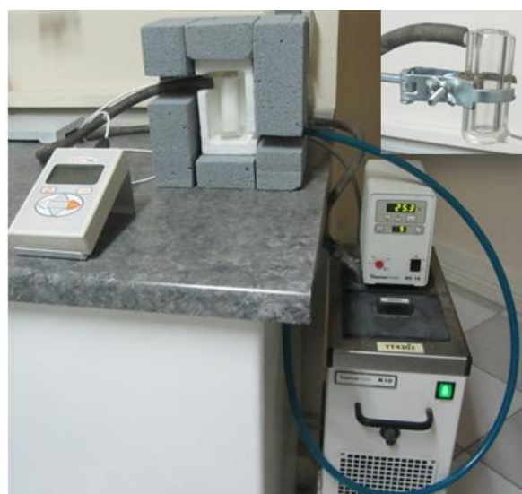
Figure 1. Experimental set up (KD2 Pro device) for thermal conductivity measurements.
