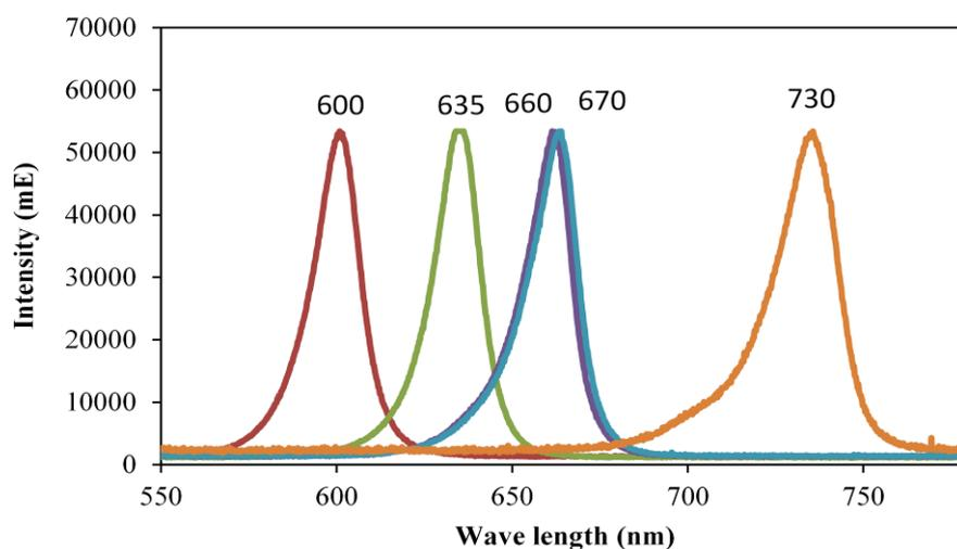
**Figure 2.** The spectral irradiance of each wavelength used in chemostat setup.
