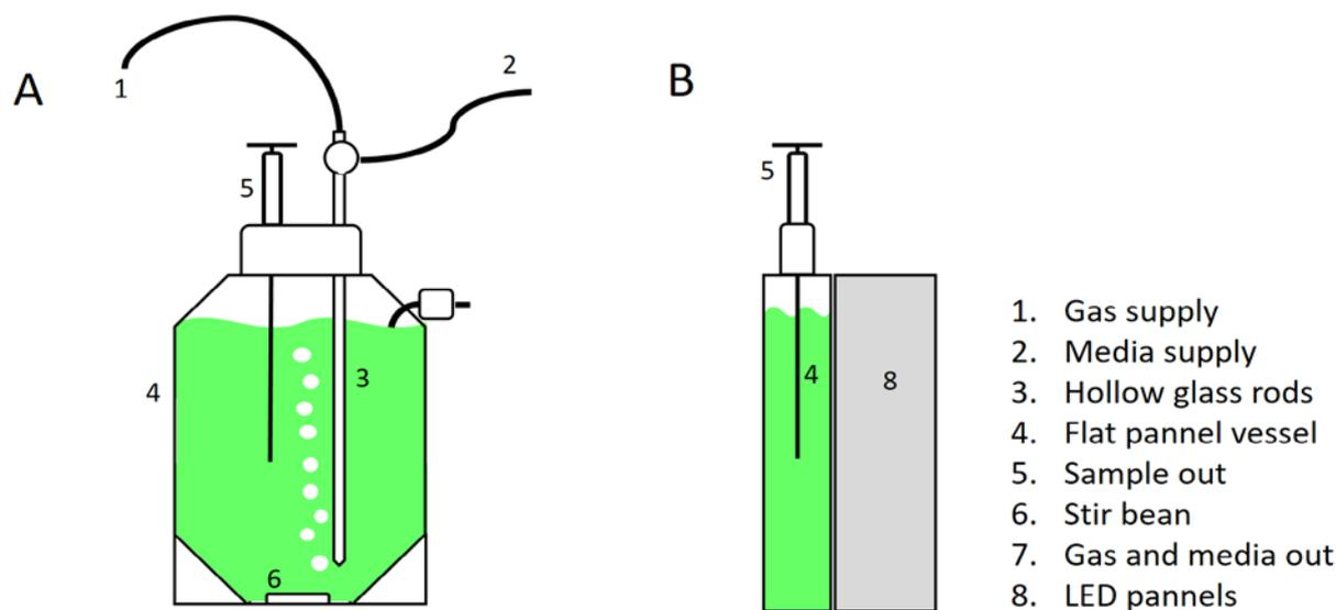
**Figure 1.** Schematic diagram of the photobioreactor used for chemostat experiments: a) front view, b) side view.
