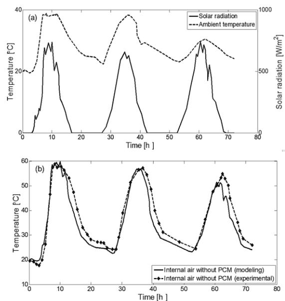
**Figure 14.** (a) Solar radiation and ambient temperature variations and (b) comparison between theoretical and experimental values for internal air without using PCM.
