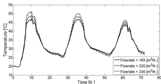
**Figure 17.** Effect of mass flow rate on internal temperature.
