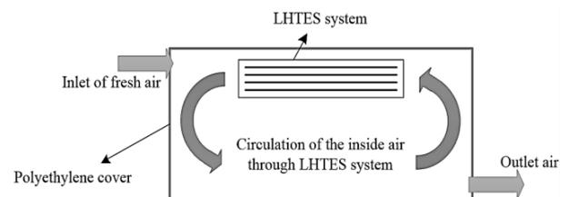
**Figure 1.** The schematic figure of the greenhouse.
