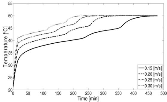
**Figure 9.** Temperature distribution of the hot cycle at different mass velocities.
