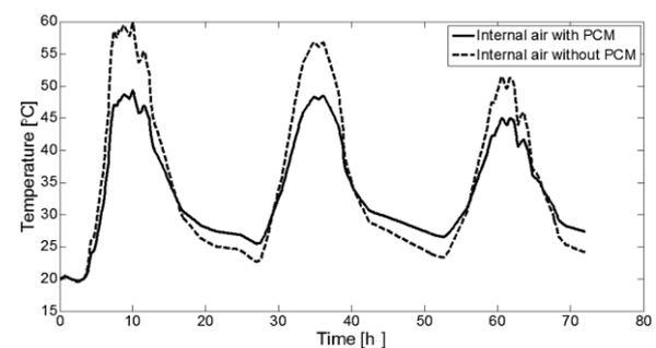
**Figure 16.** Comparison of internal air with and without using PCM.
