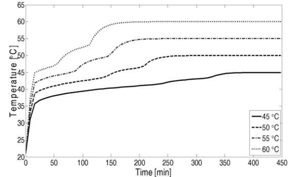
**Figure 7.** Temperature distribution of the hot cycle at different inlet temperatures.
