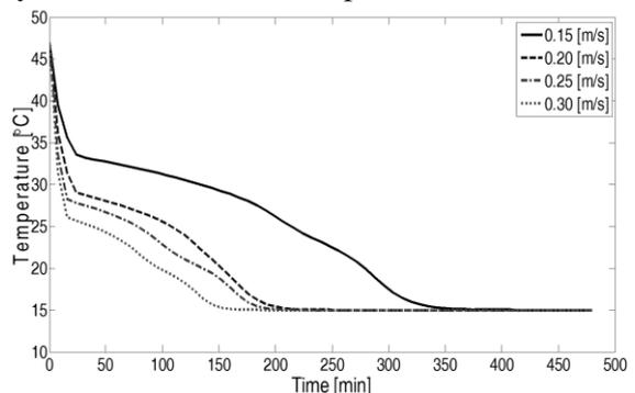
**Figure 8.** Temperature distribution of the cold cycle at different inlet air velocities.
