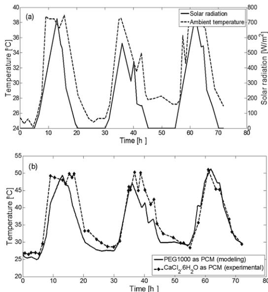
**Figure 15.** (a) Solar radiation and ambient temperature variations and (b) comparison between theoretical and experimental values for internal air using PCM.
