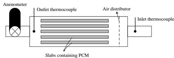
**Figure 3.** The schematic diagram of the built LHTES system.
