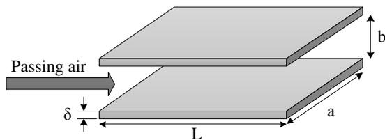
**Figure 2.** Configuration of the PCM slabs for establishing the energy balance equation.
