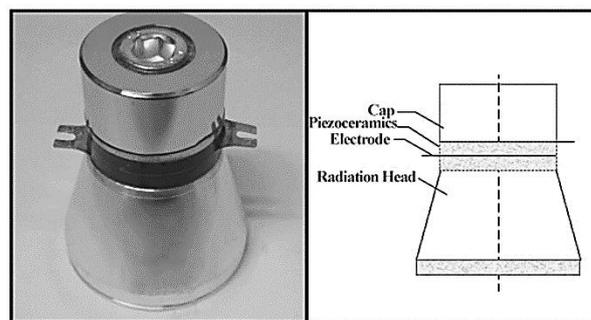
**Figure 2.** 25 KHz 100W Ultrasonic Transducer (A) real (B) schematic.
