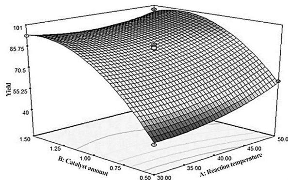
Figure 5. Response surface of yield of biodiesel vs. reaction temperature and catalyst amount.
