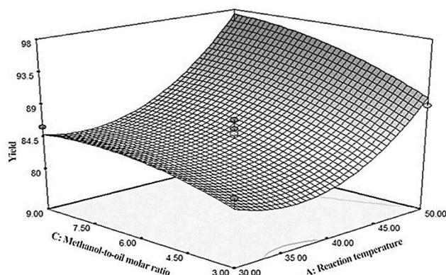
**Figure 6.** Response surface of yield of biodiesel vs. reaction temperature and methanol-to-oil molar ratio.
