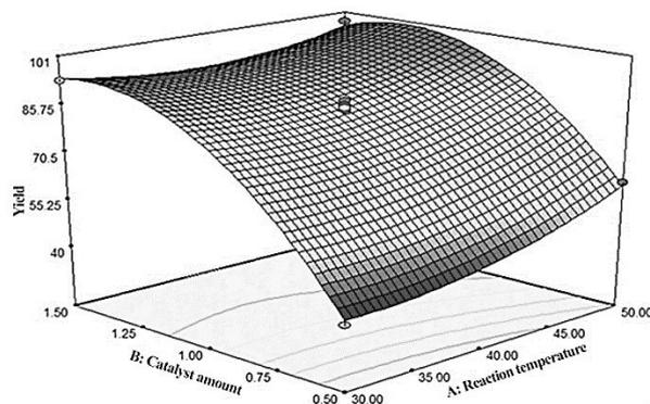
Figure 5. Response surface of yield of biodiesel vs. reaction temperature and catalyst amount.
