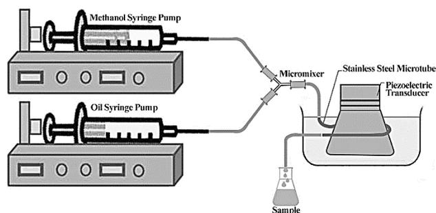
**Figure 3.** A schematic view of the experimental reaction setup.
