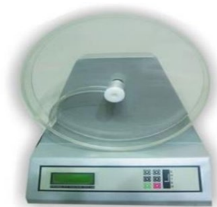
Figure 3. Friabilator device used to measure the SE (Surface Erosion) of tablets.
