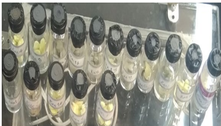
Figure 4. 16 Different types of pellets made according to the Taguchi experimental design.
