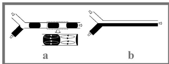
**Figure 5.** Major stable flow regimes possible for a biphasic mixture in capillary microreactors: (a) slug flow, (b) parallel flow.
