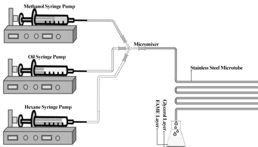
**Figure 1.** Experimental set-up of the transesterification reaction carried out in a microreactor.
