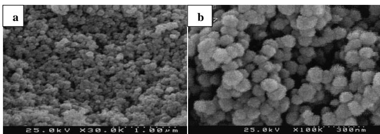
**Figure 1.** SEM images of synthesized AP-MSNs a) Resolution=30.0 k and b) Resolution=100 k.
