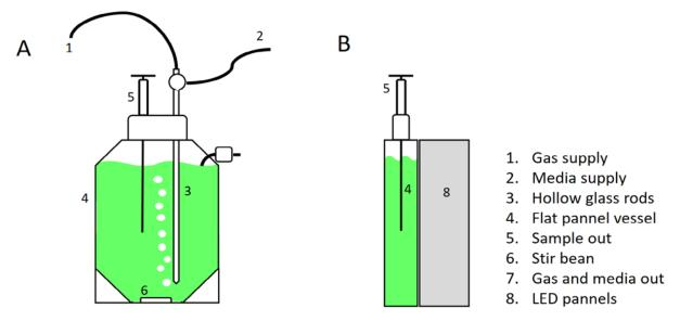
Figure 1. Schematic diagram of the photobioreactor used for chemostat experiments: a) front view, b) side view.
