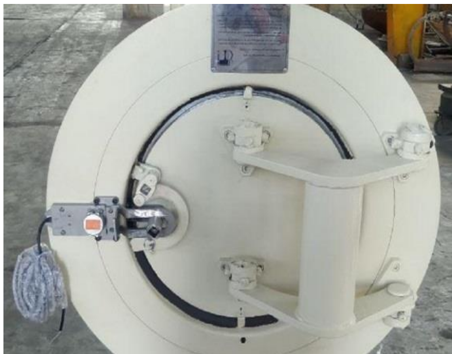
Figure 2. Filter separator lid for the cartridge replacement.
