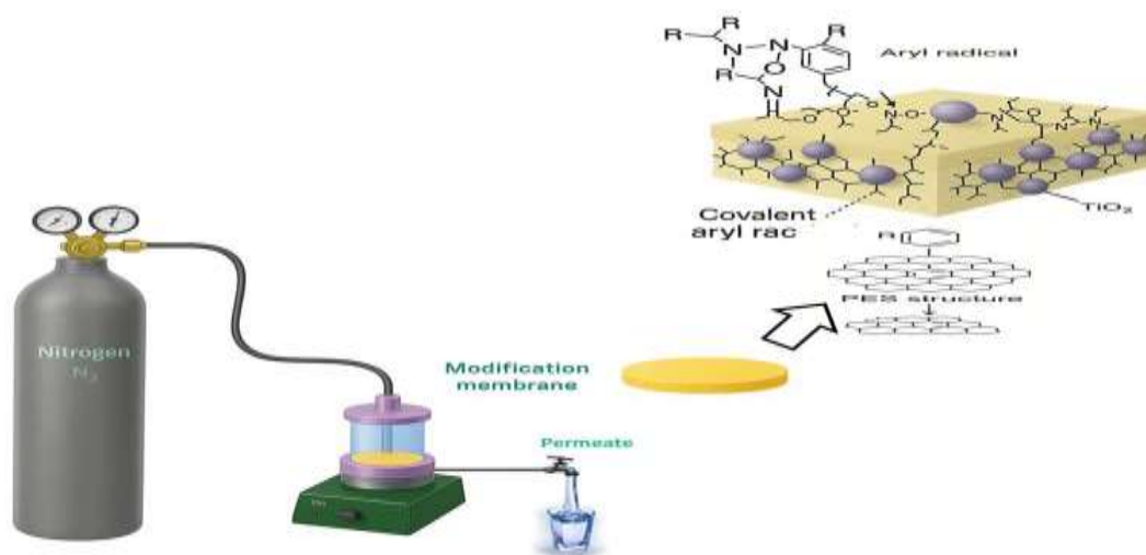
Figure 1. View of the dead-end laboratory system and the structure of the modified PES NF/TiO 2 /AO membrane.
