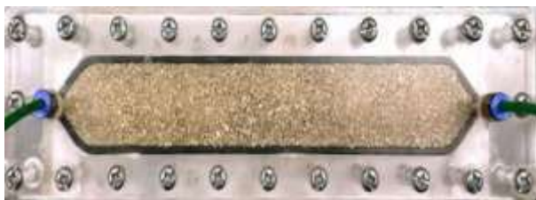
Figure 1. Schematic of the simulated two-dimensional micro-bed composed of carbonate rock grains
