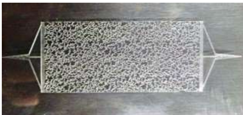
Figure 2. Two-dimensional glass micromodel used for oil recovery tests. The micromodel was treated with a mixture of 2 wt% silane and 98 wt% toluene to create oil-wet conditions, simulating a reservoir environment for evaluation. This treatment provides a realistic representation of reservoir wettability, which is critical for assessing the effectiveness of nanofluids under conditions that mimic actual subsurface formations.
