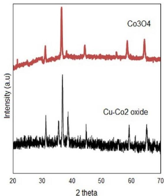
**Figure 1.** XRD pattern of Cu-Co<sub>2</sub> oxide and Co<sub>3</sub>O<sub>4</sub>.
