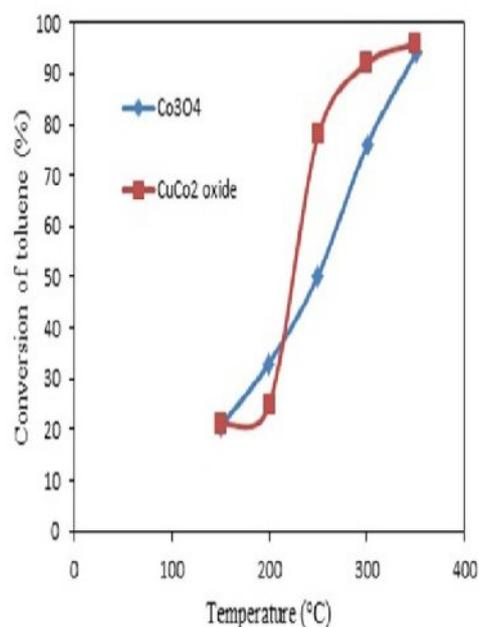
**Figure 6.** Light-off curves for catalytic conversion of toluene over catalysts.
